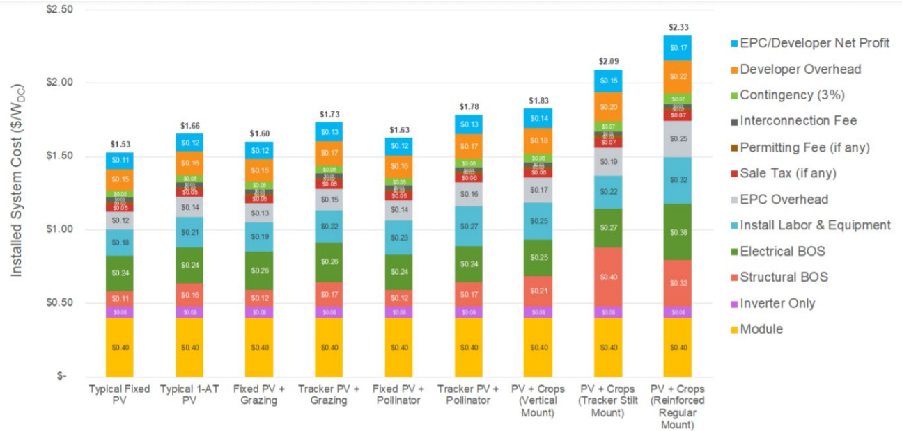
Figure 3. PV installed system costs for each dual-use scenario with benchmark assumptions for a PV system with 500 kW rated power
