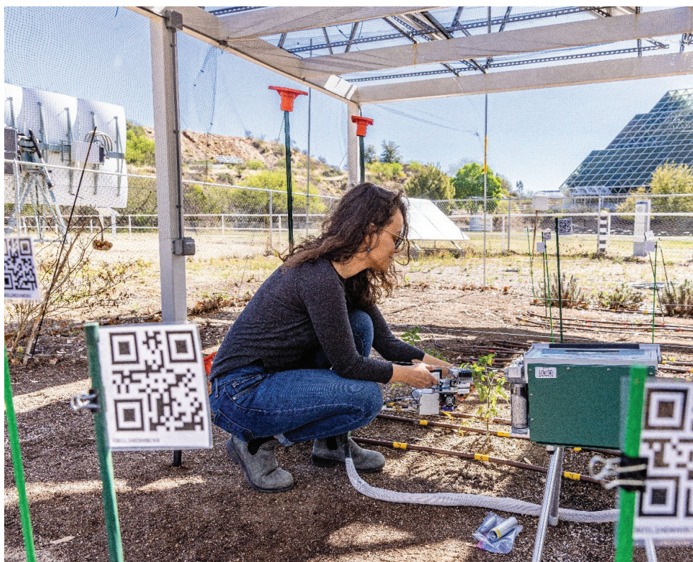
Sensors measuring soil moisture, plant, and microclimate conditions at Biosphere Agrivoltaic Site in Oracle, Arizona. Photo: AgriSolar Clearinghouse
