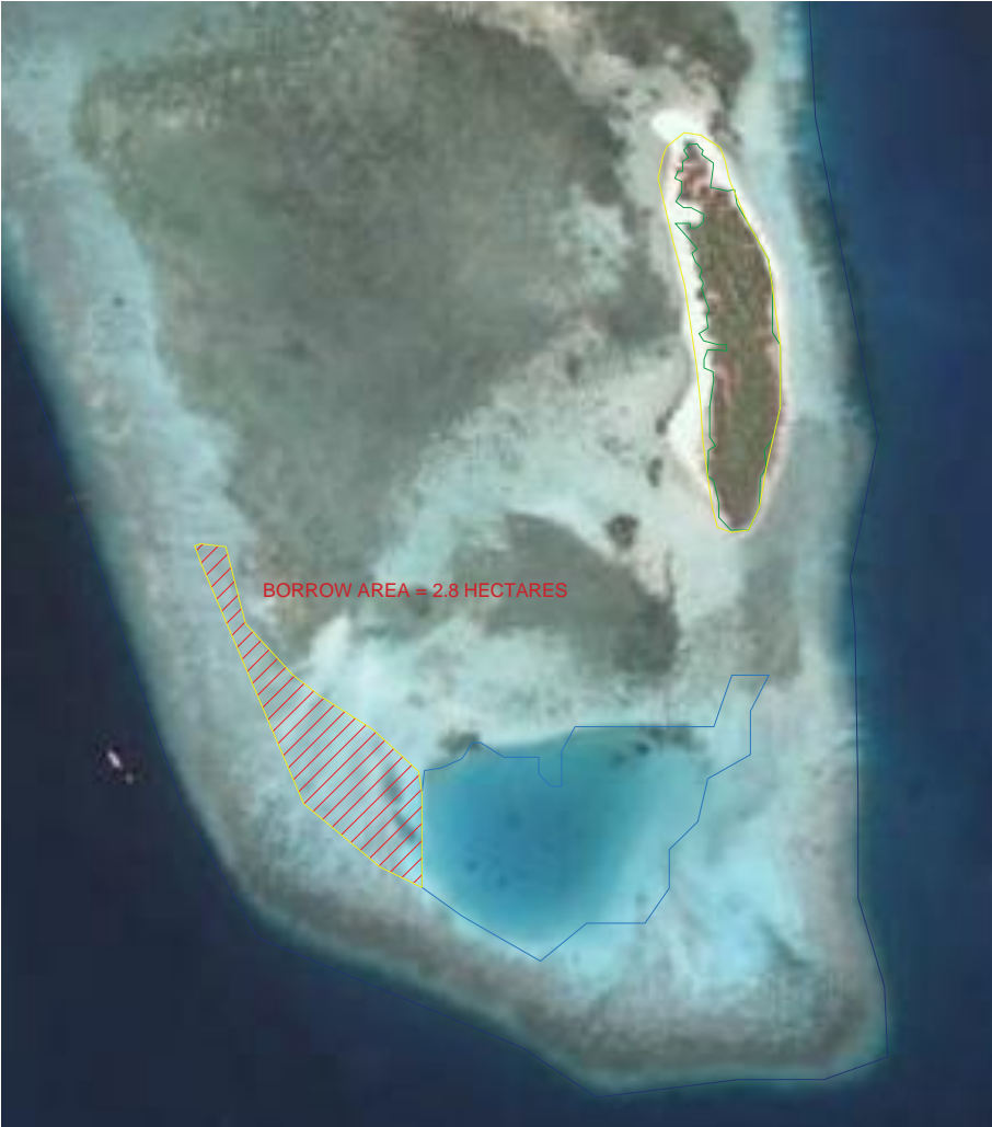
Figure 6: Location and size of the borrow area.
