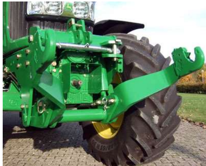
Figure 1. PTO shaft output of a tractor, source: http://www.fronthitch.com
