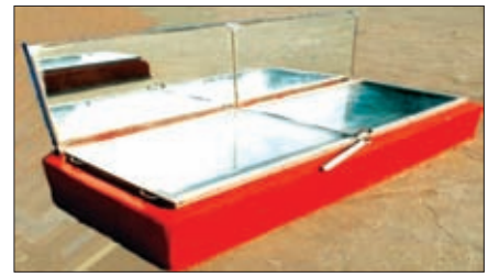
Fig. 6. Solar cooker for animal feed with reflector
