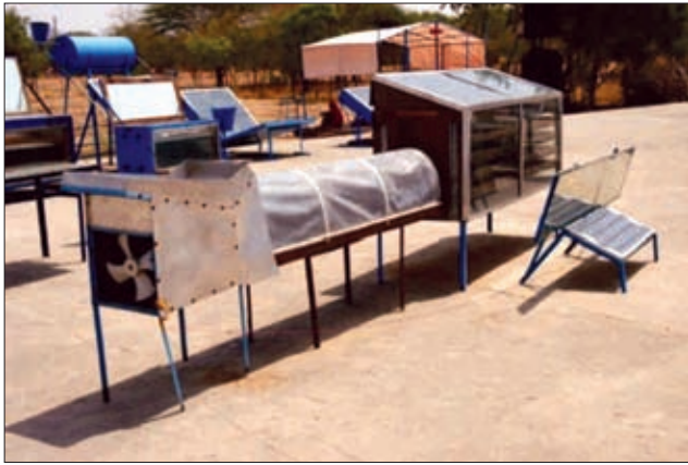
Fig. 5. Photovoltaic winnower-cum-solar dryer
