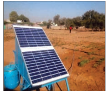
Fig. 2. Solar photovoltaic sprayer
