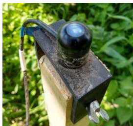
Figure 8: PAR sensors to measure the change in solar radiation below the PV modules
