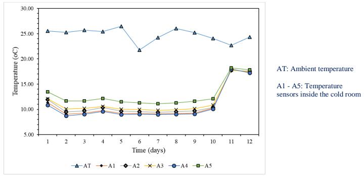
Figure 7-2: Temperature inside the cold storage as a function of time
