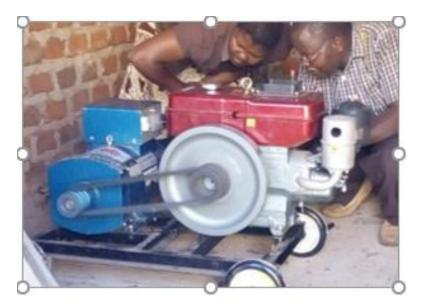
Figure 6-3: Affordable diesel engine with an alternator.
