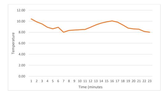
Figure 7-3 Temperature changes inside the cold room
