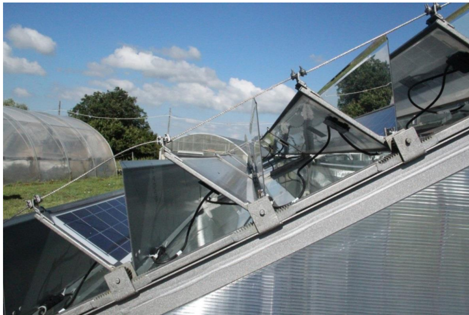
Figure 7. Detail of the movement system of the PV panels and mirrors.
