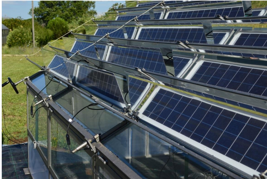
Figure 6. PV panels and mirrors on the prototype.
