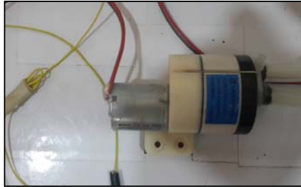
Figure 3. DC Pump used for Irrigation.
