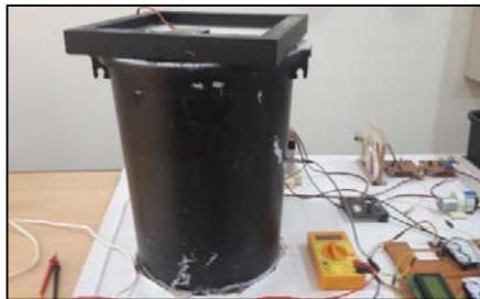
Figure 5. Fake Sun setup enclosing two incandescent bulbs and solar panel at top of the bucket.
