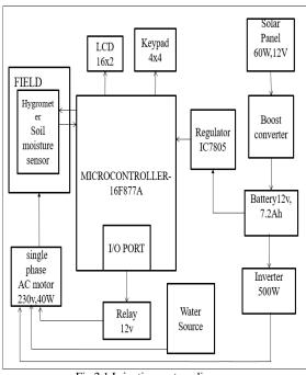
Fig 2.1 Irrigation system diagram
