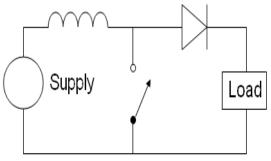
Fig: 2.2 Basic circuit of boost converter
