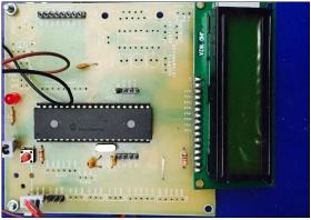
Fig 4.6 Microcontroller and LCD
