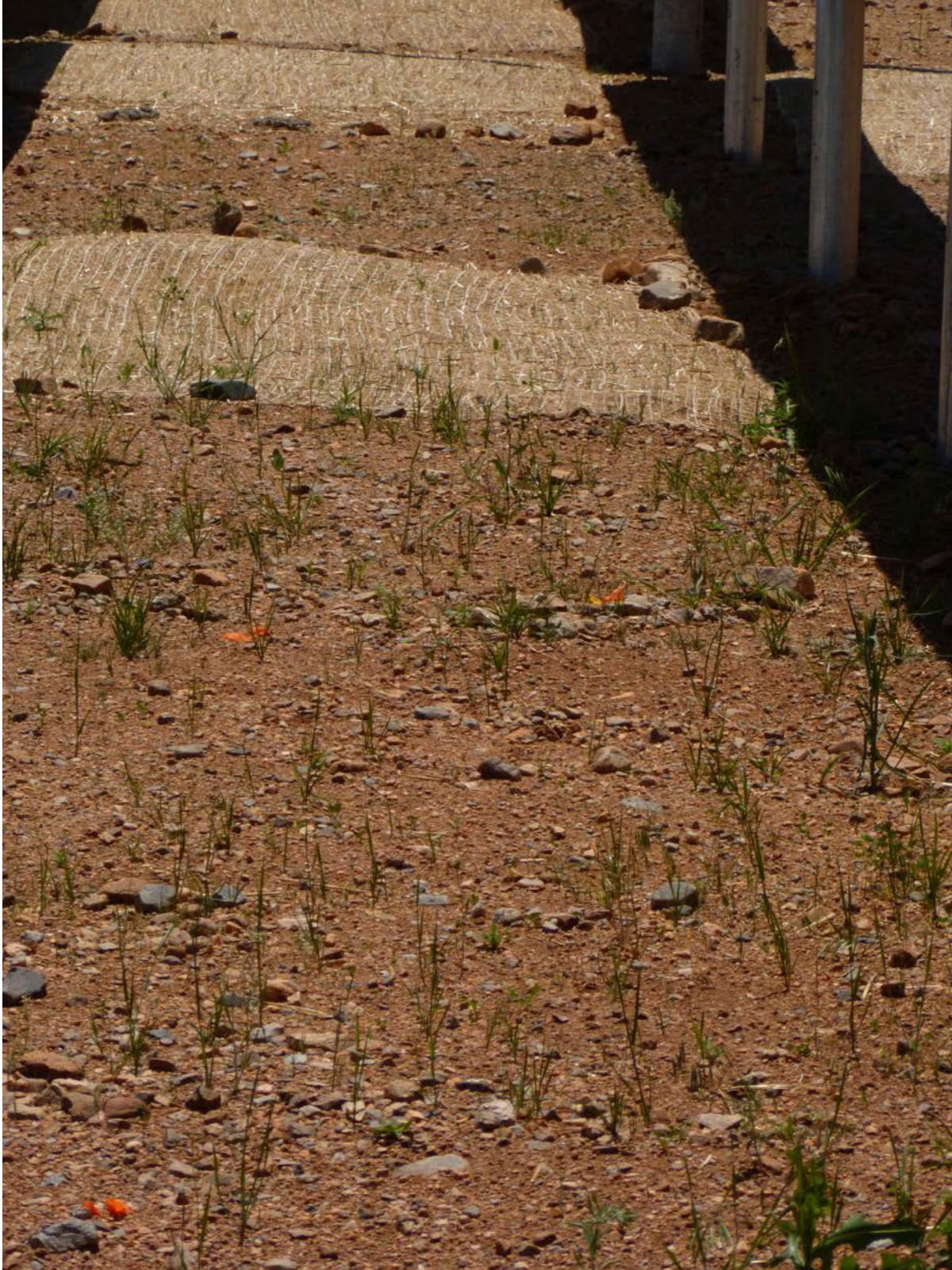
Photograph 2. Test Plots in June 2010. Foreground showing annual rye ( Lolium multiflorum ) nurse crop (A2); Midground showing matting treatment (A3); Background showing bare treatment (A1). Photo Credit: Dave Buckner
