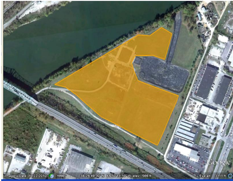
Figure 3. Partially capped north site: Recommended PV system placement Base image courtesy of Google Earth
