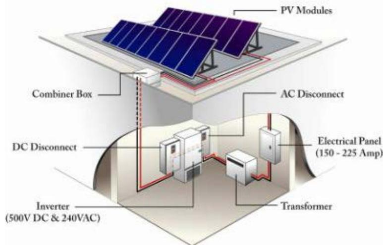
**Figure 1. Major components of grid-connected PV system**
