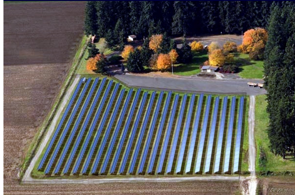
Two views (an aerial view and a view from the adjacent residential neighborhood located higher up the bluff) of the conceptual layout for the world's largest roadside solar installation, a 3 megawatt system at a maintenance and storage facility along Interstate 205 near the City of West Linn, Oregon.
