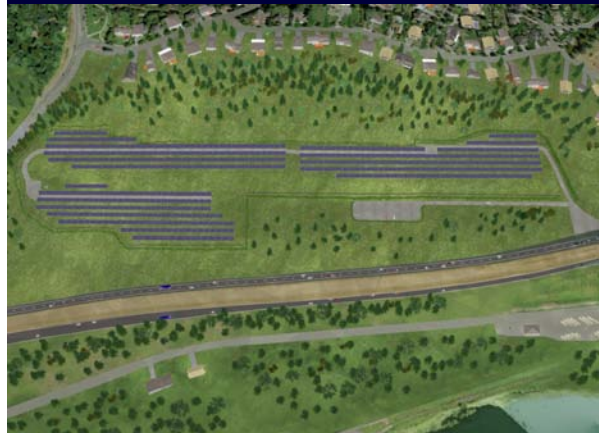
Two views (an aerial view and a view from the adjacent residential neighborhood located higher up the bluff) of the conceptual layout for the world's largest roadside solar installation, a 3 megawatt system at a maintenance and storage facility along Interstate 205 near the City of West Linn, Oregon.
