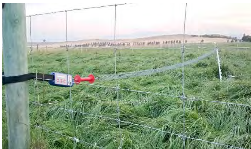
A Batt Latch is a solar-powered automatic gate opener developed in New Zealand. It retails for about $400. You can set the time when the latch will open. Livestock quickly become accustomed to the opener and move into the new paddock when it releases the spring gate. For a demonstration video, see https://www.youtube.com/watch?v=pep4aH1U3Ns . Photo: Dave Scott, NCAT
