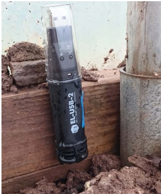
Easy Log – USB data loggers were placed in both tunnels and outside. Photo: Chris Lent, NCAT
