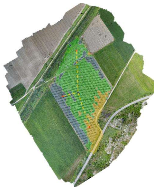
Figure 8. Sensor nodes positioning based on the zones defined by performing fuzzy clustering on the soil ECa, surface elevation data, and the field's topology environment.
