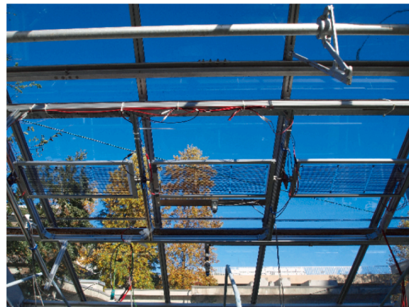
Fig. 7. Prototype PV blind system installed underneath the experimental greenhouse glass roof facing the eastern sky.
