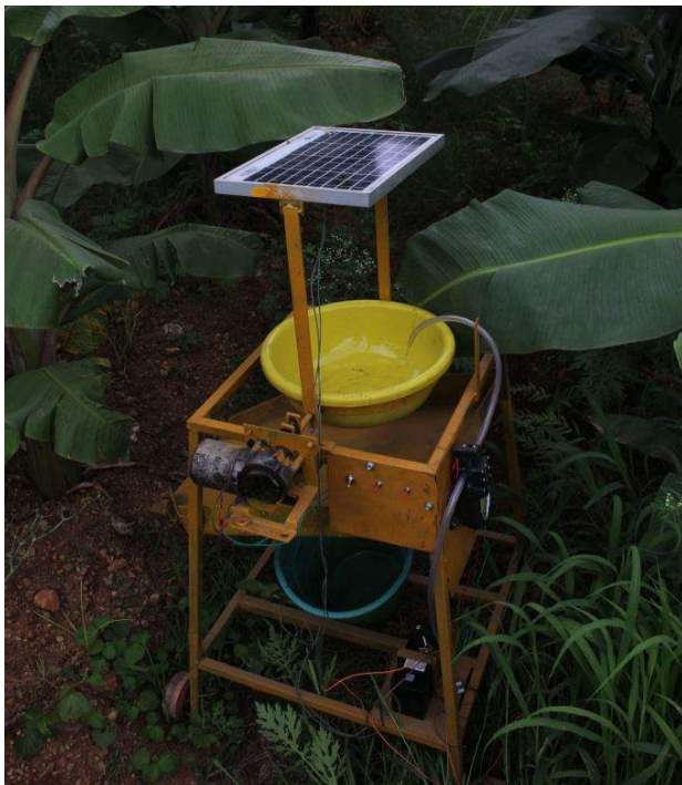
Fig-13: Automated refilling of water to basin
